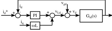
Figure 7. Current control loop (d-component)
