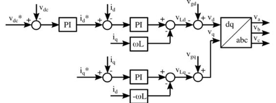
Figure 4. Decoupled control diagram.
