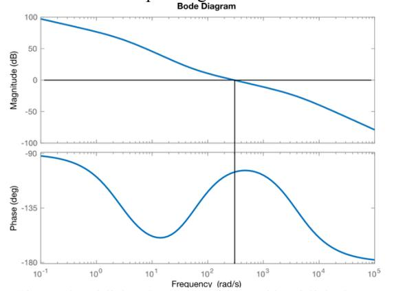
Figure 10. DC link voltage control loop with DC link plant.
