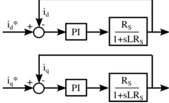
Figure 8. Current control loop with filter plant.
