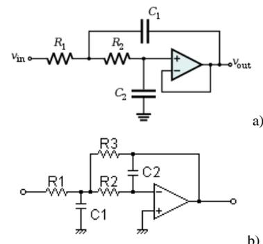
Figure 1.a) Sallen-key filter. b) Multiple feedback filter.
