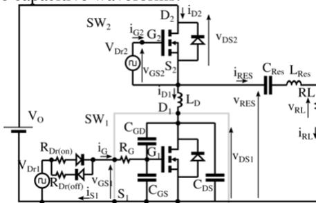
Figure 19 Diagram of RLC series resonant circuit
