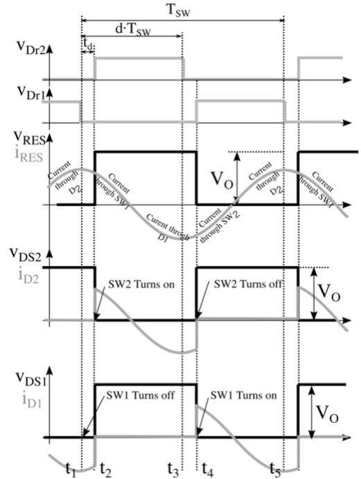
Figure 21 Waveforms in resonant circuit, for capacitive behavior
