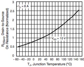
Figure 6 Normalized On-Resistance vs. temperature
