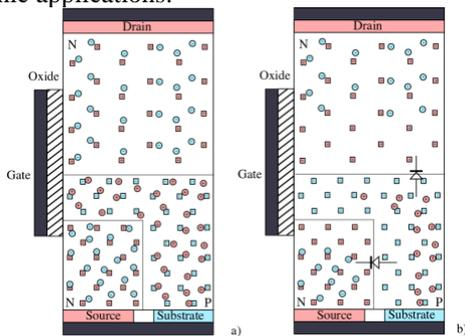
Figure 1 Structure of a standard MOSFET.
