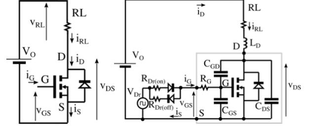
Figure 8 Equivalent circuit of the MOSFET and driver for resistive switching. Left: references at the main devices. Right: Detailed model of the switch and driver.
