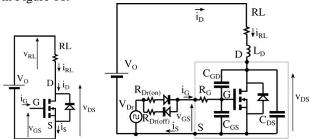
Figure 16 Circuitual model in case of resistive switching.
