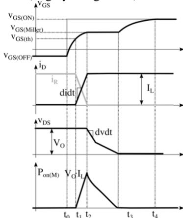
Figure 12 Waveforms at turn on (ideal rectifier diode).
