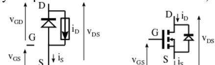
Figure 5 a) Simplified equivalent circuit of the MOSFET. b) Symbol of the N-Channel enhancement MOSFET.
