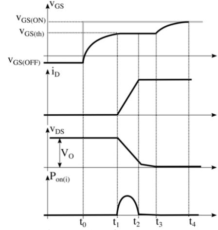
Figure 17 Waveforms at turn on.
