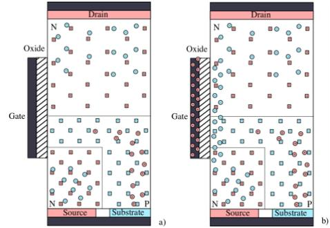
Figure 2 A N-channel MOSFET, in the off-state (a) and with a gate voltage (b). A channel of n carriers appears between drain and source.
