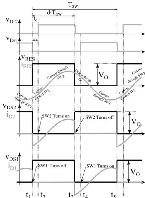
Figure 20 Waveforms in resonant circuit, for inductive behavior.
