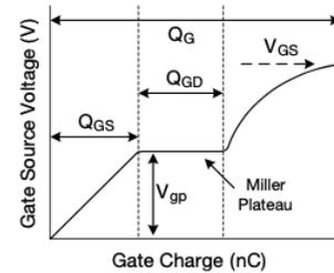
Figure 13 Gate charge as a function of the gate to source voltage, as predicted in [7].
