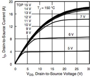
Figure 7 Typical Output characteristics
