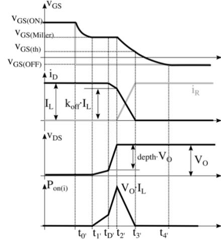
Figure 15 Waveforms at turn off.
