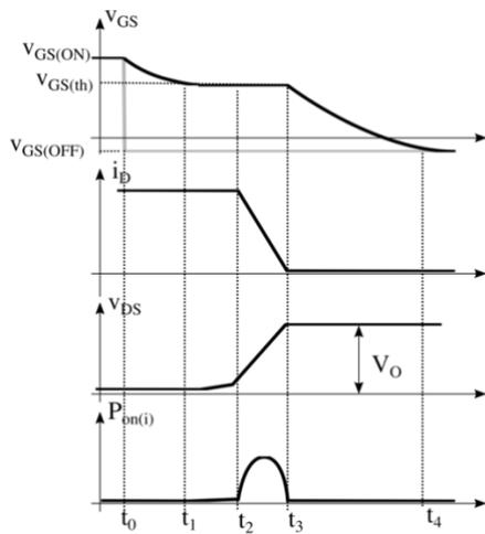
Figure 18 Waveforms at turn off.
