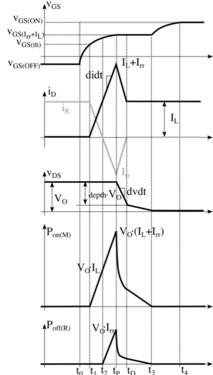
Figure 14 Waveforms at turn on (real rectifier diode).
