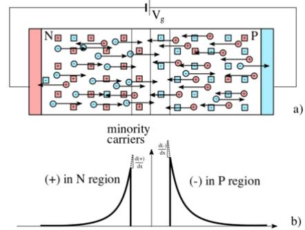
Figure 5 a) Forward bias. b) Distribution of minority carriers in steady state.
