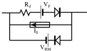
Figure 7 Static Characteristic of a real diode.
