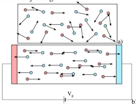
Figure 1 Intrinsic silicon scheme. a) Random movement due to temperature (any instant concentration mismatch is compensated through diffusion processes). b) Movement due to an external field.
