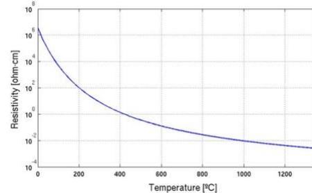
Figure 2 Variation of silicon resistivity vs. temperature [2]
