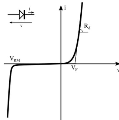
Figure 6 Static Characteristic of a diode.
