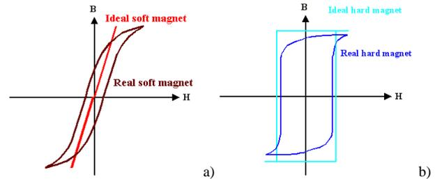
Figure 2.a) Soft Magnet. b) Hard magnet. [3]
