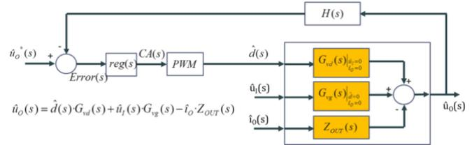
Fig. 2. Control System Block Diagram with single regulator.
