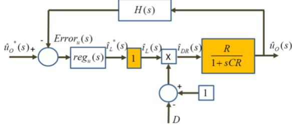
Fig. 4. Output voltage control loop
