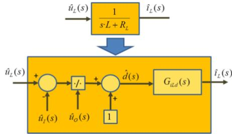
Fig. 5. Implementation of control loops – calculation of duty ratio
