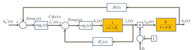
Fig. 3. Control System Block Diagram with two nested control loops
