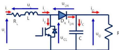
Fig. 1. Power stage of a boost converter, with voltage and current references.
